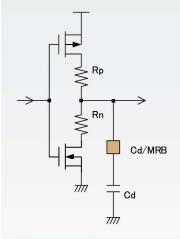
The release delay is set by Rp and Cd and the detect delay time is set by Rn and Cd. The release delay allows you to start up correctly and the detect delay avoids any misdetection due to noise and spikes. The XD6132/33/34 has five (5) different ratio configurations of Rp and Rn to fit any requirement.
