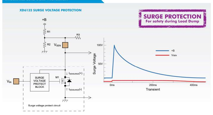
Even if 100V Load dump surge comes to +B, the internal surge voltage protection circuit protects the VSEN pin. When the surge comes and the VSEN voltage rises, the "SURGE VOLTAGE PROTECT BLOCK" detects it and turns on M1 which sinks 2.5mA and this current causes a voltage drop on R1 to keep VSEN safe.
